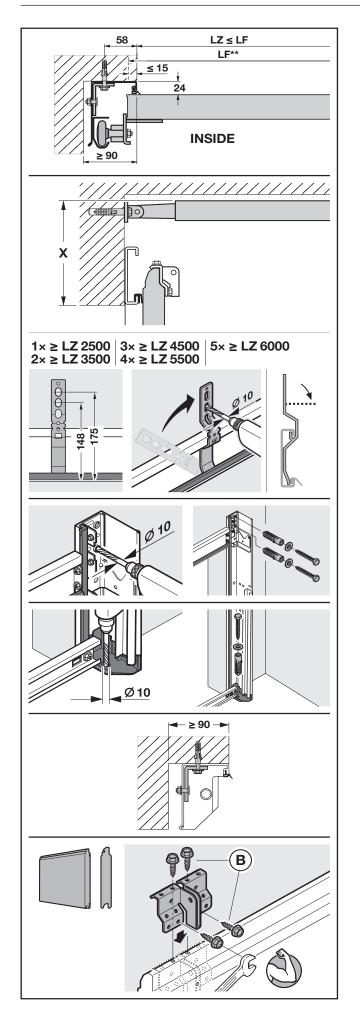
Frame legs must be fitted behind the reveals with a centreline for the fittings at 58mm from the edge of the structure.
