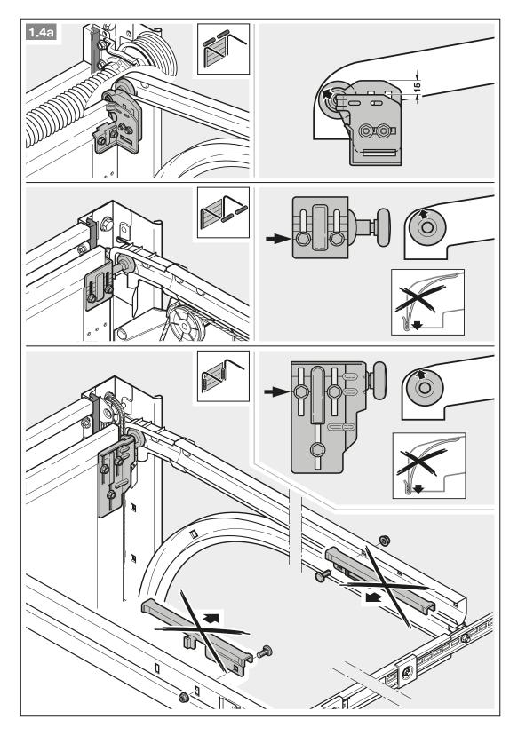
For sectional doors with central door locking, fit the lintel joint and link bracket off-centre (max. 500 mm).
